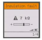
The Bender iso685 utilizes the latest in monitoring technology to detect ground faults in ungrounded AC/DC systems, as well as systems with variable frequency drives (VFD). The iso685 monitors the system's insulation resistance, and alarms when a breakdown is detected. Troubleshooting equipment has never been easier with the new isoGraph feature, which trends the system's insulation resistance over time.
