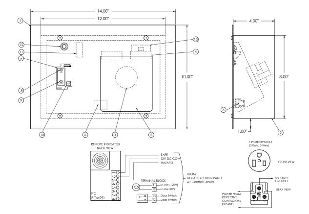
Sample outline: XRM module with MK2000 remote indicator and in-use lamp (example part number: XRM-5B2)
