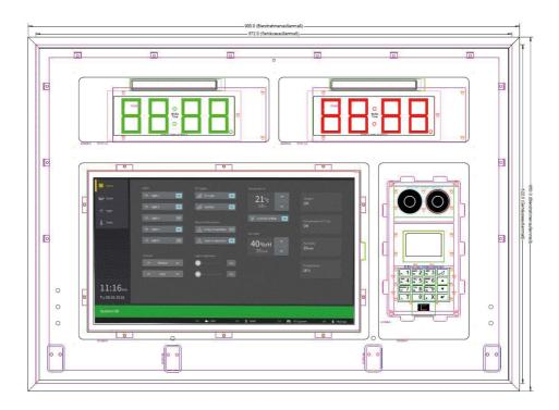
Fig. 2–2 CP921-F in bezel frame enclosure with individual, project-specific internal components
