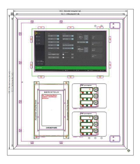
Fig. 2–1 CP915-F in bezel frame enclosure with individual, project-specific internal components
