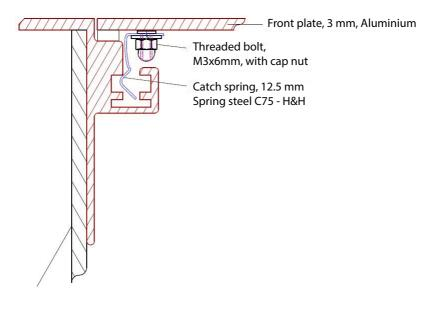
Fig. 3–1 Cross section view
