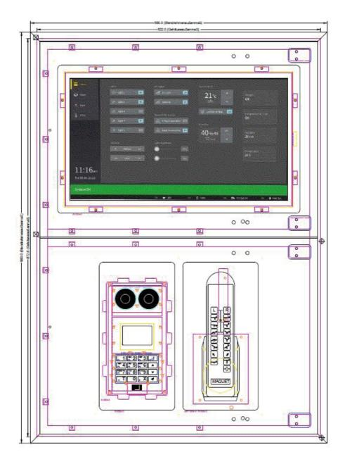
Fig. 2–3 CP921-F with two front plates in bezel frame enclosure. Lower front plate with individual, project-specific internal components
