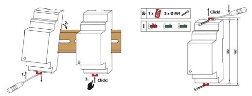
Figure: DIN rail mounting (left) or screw mounting (right)
