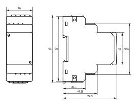
Figure: Dimension diagram (in mm)
